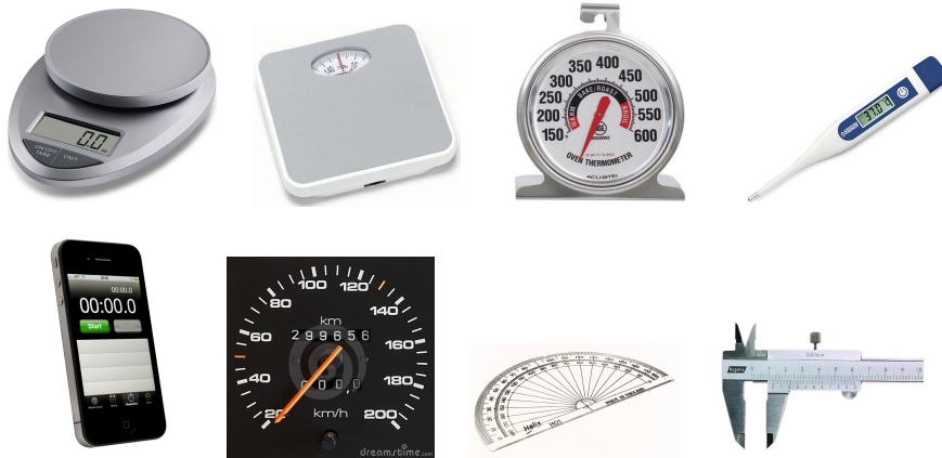
kitchen scale, person scale, thermometer (oven), thermometer (medical), stopwatch, speed meter, protractor, vernier scale
